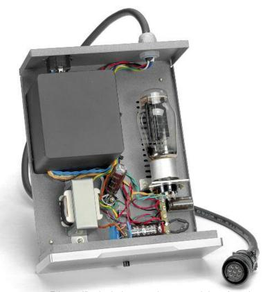
Tube rectification in the external power supply is performed by a powerful Russian military stock 5AR4 tube. The physical separation of electronics and power supply allows the use of a particularly powerful transformer. The influence of magnetism or vibrations can thus be practically ruled out. Partnering equipment:Turntables: Nottingham Analogue Dais including Sperling Audio NRM-1/S motor housing, Pear Audio Blue Little John
