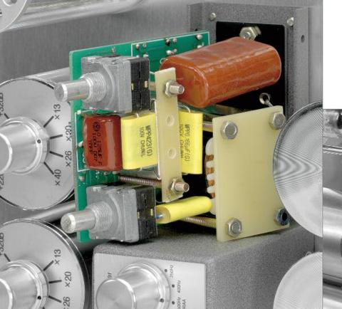
Left and below: The passive RIAA equalization is achieved via an LCR network (L = inductance of the coil/C = capacitance of the capacitor/R = resistance) and has a special feature: the capacitor is not located in the signal path, but is connected in parallel. Kang Su Park's circuit designs always involve very careful component selection
